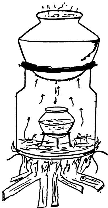
Fig 7. Raksi distillation apparatus showing distillate being collected into a small metallic vessel kept above tripet-stand inside the main cylindrical container
