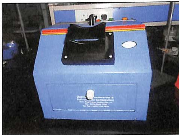
Fig 3.6: UV Fluorescence Analysis Cabinet
