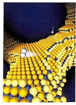
Controlling surface structure at the atomic scale is paramount to developing effective catalysts. The surface structure of MoS<sub>2</sub> is now engineered to preferentially expose edge sites by successfully synthesizing contiguous largearea thin films of a highly ordered double-gyroid MoS<sub>2</sub> bicontinuous network with nanoscale pores. (Image: © Jakob Kibsgaard, Zhebo Chen and Thomas F. Jaramillo)
