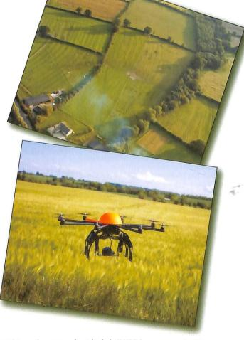
**Cover picture:** An unmanned aerial vehicle (UAV) known as an octocopter surveys an agricultural landscape. Recent technological improvements are allowing UAVs equipped with various remote-sensing instruments to collect ecological data at fine spatial and temporal resolutions.
