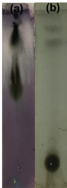
Figure 6.27: TLC plates for methanol extract of Acacia concinna derivatized with anisaldehyde-sulphuric acid reagent using (a) (Chloroform: Glacial acetic acid: Methanol: Water [8:4:1.5:1]) (b) (Petroleum ether: Ethyl acetate [80:20]).
