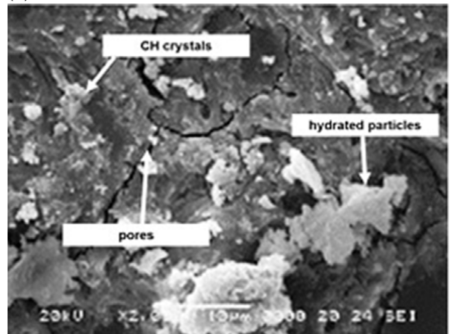
FIGURE 5 Scanning electron microscopic (SEM) photograph of (a) OPC70% + FA15% + SF7.5% + GGBS7.5% and (b) OPC70% + FA15% + SF7.5% + MK7.5%
