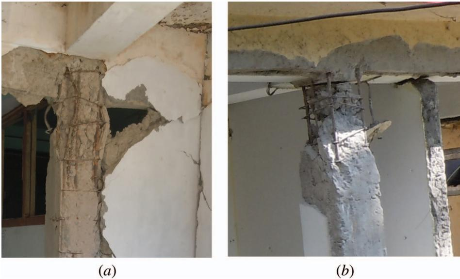
Figure 8. (a) and (b) Typical failure at column ends (widely spaced stirrups with 90° hooks, cold junction at the column top, poor concrete quality).
