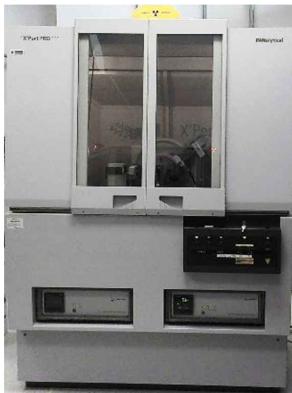
Figure B1.13: Photograph of PANalytical X-Ray diffractometer.
