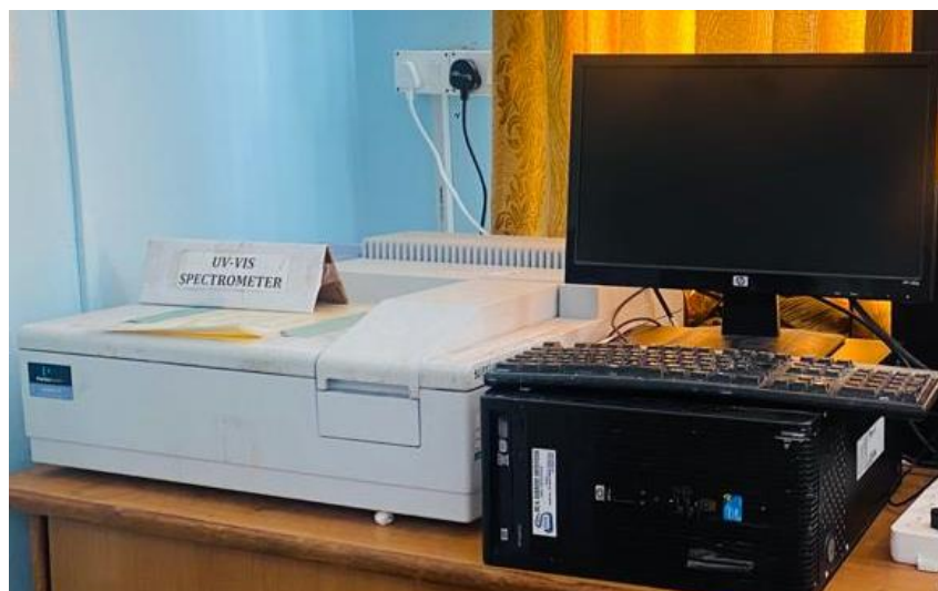
Figure B1.7: Photograph of a Perkin Elmer spectrophotometer (Range: 190-1100 nm)
