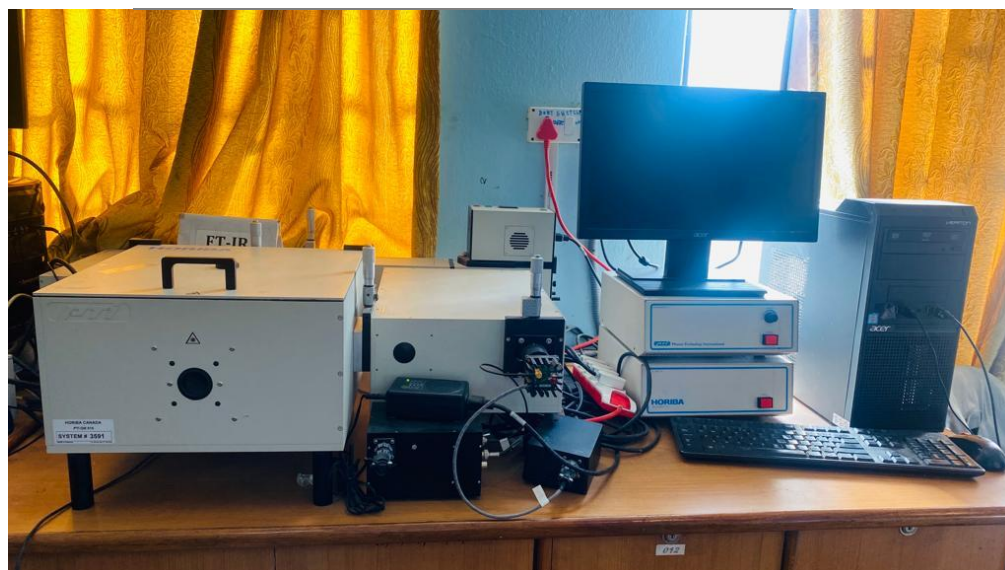
Figure B1.11: Photograph of HORIBA Scientific spectrophotometer (Model: PTI-QM 510)
